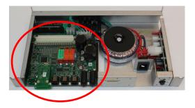
3. Install the NGMCB controller in the new NGI-85 and reinstall the retaining plate from part 1.
