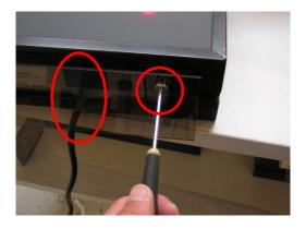
3. Remove the retaining plate holding the NGMCB controller in place.
